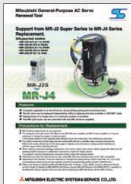
MR-J2S Renewal Tool Catalog X901307-312 This guide introduces a renewal tool for replacing MR-J2S with MR-J4. The renewal tool allows to use the existing wiring and mounting holes, making the replacement simple and fast.
