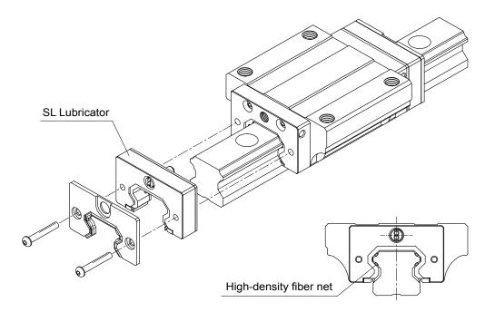
By using the SL Lubricator, the interval between maintenance work can be lengthened at all load ratings.
