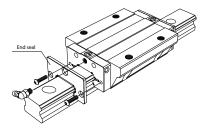
Bidirectional seal when high dust protection is required.
