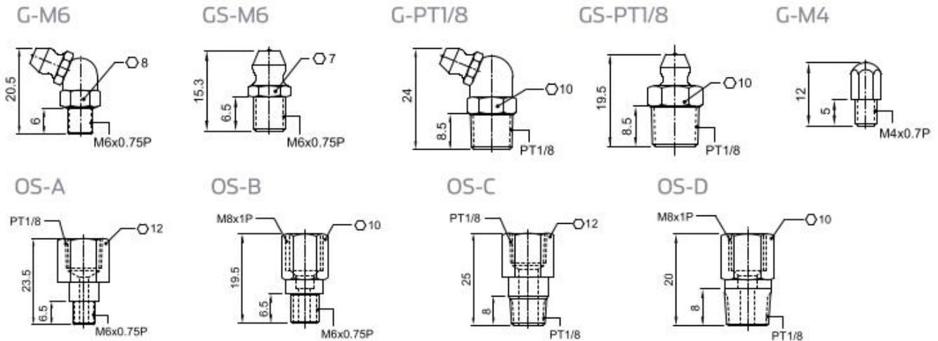
The standard mounting location on the carriage is at the center of both ends. As shown below, lubrication from the side of the carriage is achieved by using an adapter to connect the grease/oil fitting to the hole on the carriage.
