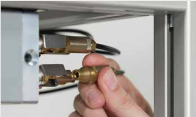
The hydraulic lines can be connected up to the pump unit in next to in time thanks to quick-action couplings.
