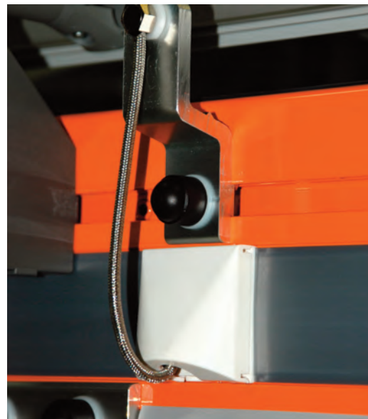
Cable raceways integral to the conveyor.
