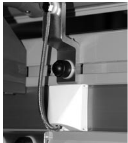
Cable raceways integral to the conveyor.
